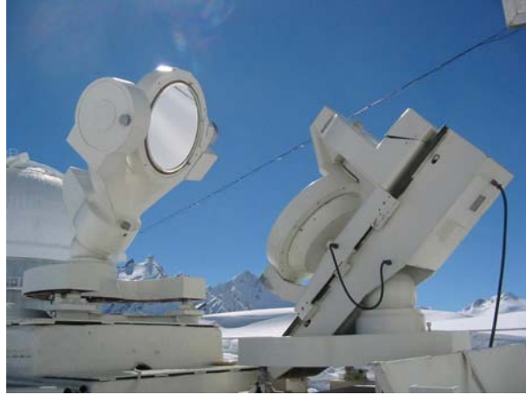
Fig. 4 The large horizontal solar telescope ACU-26
