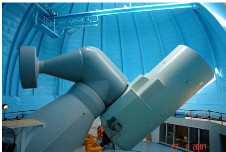
Fig. 2 The 2-m Ritchey-Chrétien Coudé telescope
